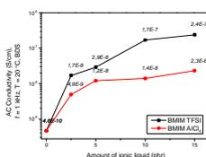
Figure 1. AC conductivity in function of IL amount in XNBR/MgAl-LDH composite.
